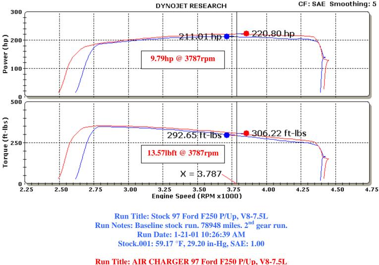
Run Notes: 63-1014 AIR CHARGER installed. 78948 miles. 2<sup>nd</sup> gear run. Run Date: 1-21-01 12:58:19 pM FIPK.002: 66.83 °F, 29.25 in-Hg, SAE: 1.01
