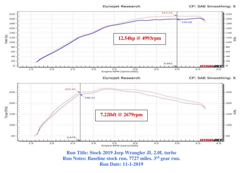
Run Title: K&N 2019 Jeep Wrangler JL 2.0L turbo Run Notes: K&N intake kit #63-1580 installed. 7727 miles. 3<sup>rd</sup> gear run. Run Date: 11-1-2019
