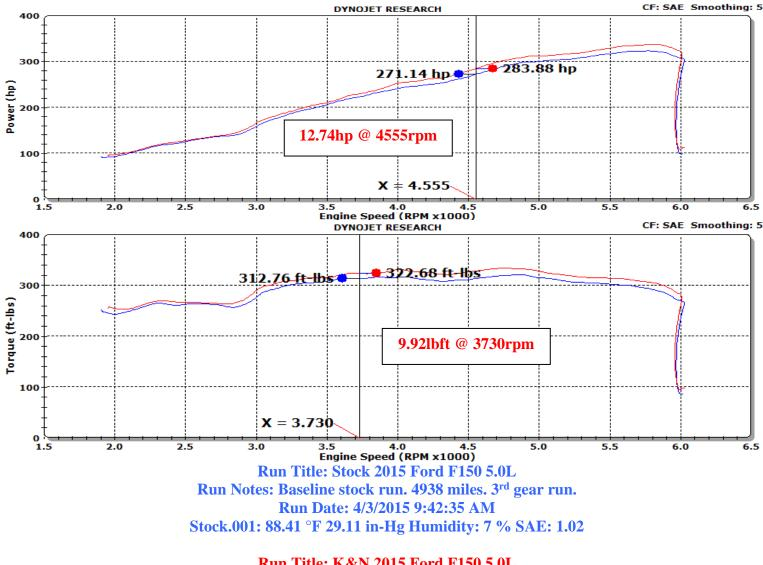
Run Title: K&N 2015 Ford F150 5.0L Run Notes: K&N intake kit #63-2591 installed. 4938 miles. 3<sup>rd</sup> gear run. Run Date: 4/3/2015 11:12:52 AM K&N.002: 88.86 °F 29.09 in-Hg Humidity: 6 % SAE: 1.02
