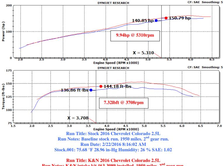
Run Notes: K&N intake kit #63-3089 installed. 1950 miles. 2<sup>nd</sup> gear run. Run Date: 2/22/2016 9:30:11 AM K&N.002: 84.41 °F 28.99 in-Hg Humidity: 8 % SAE: 1.02
