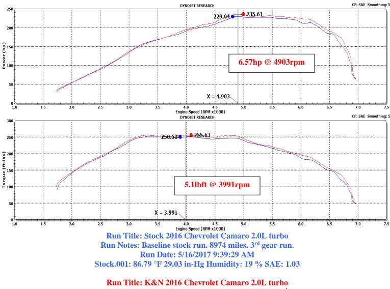
Run 11tie: K&N 2016 Chevrolet Camaro 2.0L turbo Run Notes: K&N intake kit #63-3105 installed. 8974 miles. 3<sup>rd</sup> gear run. Run Date: 5/16/2017 1:53:46 PM K&N.002: 88.67 °F 29.02 in-Hg Humidity: 19 % SAE: 1.03
