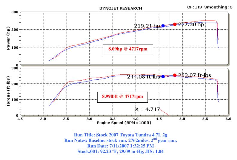
Run Title: K&N 2007 Toyota Tundra 4.7L 2g Run Notes: K&N intake kit #63-9032 installed. 2762 miles. 2<sup>nd</sup> gear run. Run Date: 7/11/2007 2:40:20 PM K&N.002: 100.40 °F, 29.05 in-Hg, JIS: 1.05
