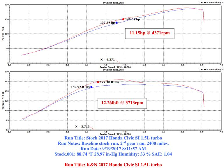
Run Title: K&N 2017 Honda Civic SI 1.5L turbo Run Notes: K&N intake kit #69-1504TR installed. 2<sup>nd</sup> gear run. 2400 miles. Run Date: 9/19/2017 9:36:20 AM K&N.002: 91.25 °F 28.98 in-Hg Humidity: 28 % SAE: 1.04
