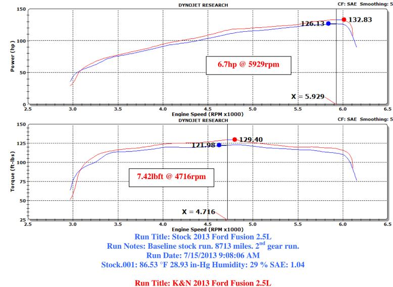
Run Title: K&N 2013 Ford Fusion 2.5L Run Notes: K&N intake kit #69-3533 installed. 8713 miles. 2<sup>nd</sup> gear run. Run Date: 7/15/2013 10:16:14 AM K&N.002: 89.32 °F 28.95 in-Hg Humidity: 22 % SAE: 1.04
