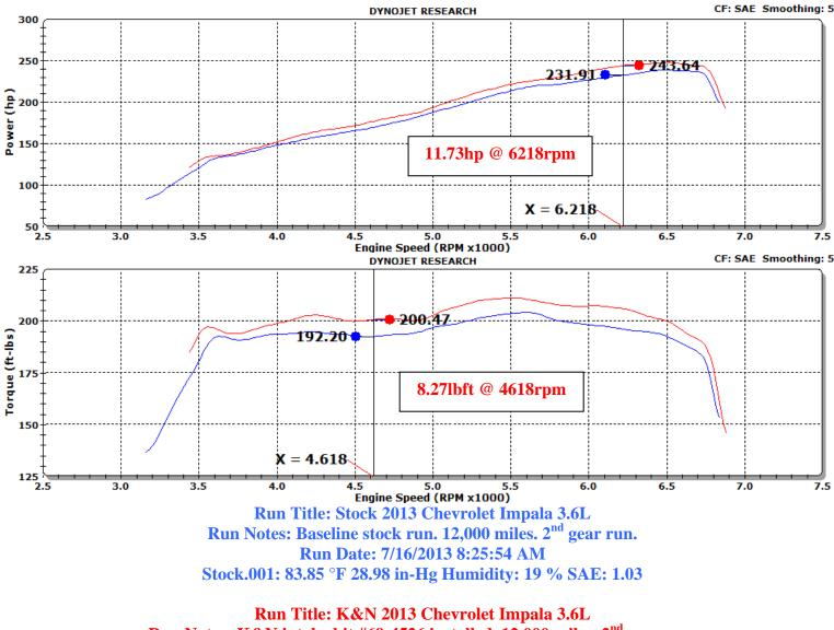
Run Title: K&N 2013 Chevrolet Impala 3.6L Run Notes: K&N intake kit #69-4526 installed. 12,000 miles. 2<sup>nd</sup> gear run. Run Date: 7/16/2013 9:27:51 AM K&N.002: 85.46 °F 28.97 in-Hg Humidity: 17 % SAE: 1.03
