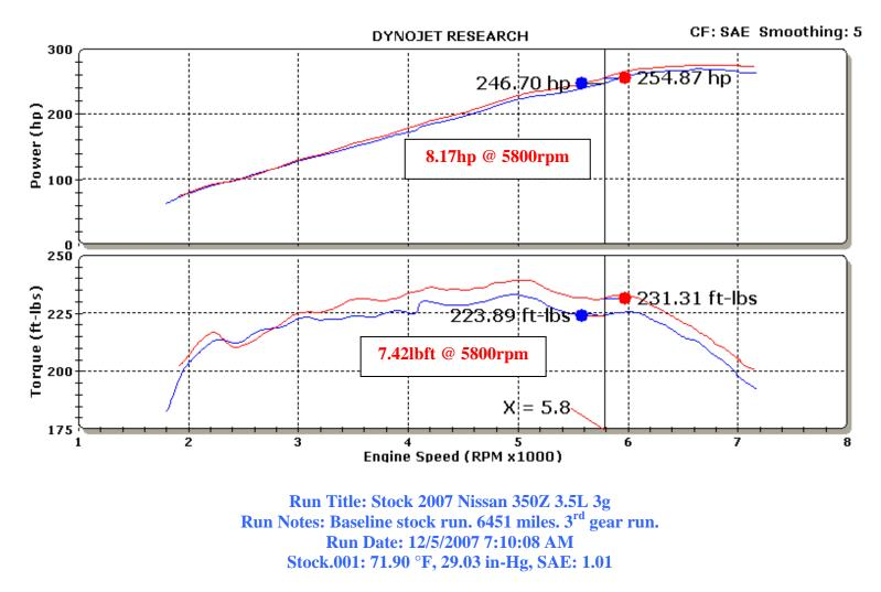
Run Title: K&N 2007 Nissan 350Z 3.5L 3g Run Notes: K&N intake kit #69-7071 installed. 6451 miles. 3<sup>rd</sup> gear run. Run Date: 12/5/2007 10:01:33 AM K&N.002: 81.54 °F, 28.99 in-Hg, SAE: 1.02
