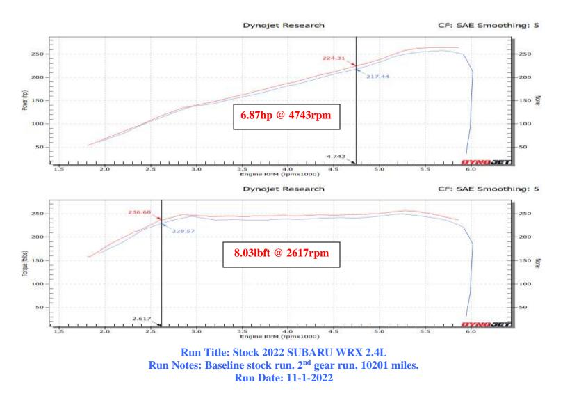
Run Title: K&N 2022 SUBARU WRX 2.4L Run Notes: K&N intake kit #77-1017C installed. 2<sup>nd</sup> gear run. 10201 miles. Run Date: 11-1-2022
