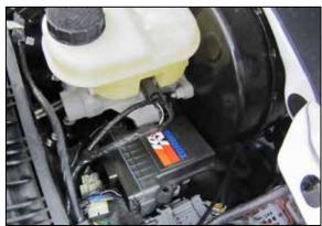
5. Mount the boost module in a suitable location such as under the brake master cylinder as shown using the provided tie wraps.
