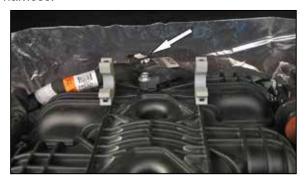
3. Remove the engine cover and then disconnect the MAP sensor electrical connection at the rear of the intake manifold.
