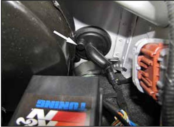
7. Poke a small hole in the existing firewall grommet and feed the boost control knob wiring harness through the grommet from the inside of the vehicle. Connect the control knob wiring harness to the pigtail connected to the module. And secure with the provided tie wraps.
