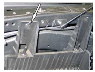
17. Remove the front air box mounting bracket bolt shown. **NOTE: This bolt will used in a later step.**
