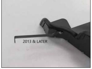
16. Install the heat shield mounting bracket (008103-1) onto the heat shield using the provided hardware. **NOTE: Do not completely tighten at this time.**
