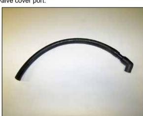
8. Remove the factory 45 deg. elbow from the factory ccv hose assembly. Assemble the K&N CCV hose, union and factory 45deg. elbow as shown.
