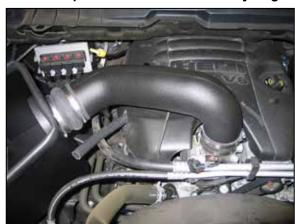
25. Install the K&N intake tube into the silicone hump hose and then into the silicone hose at the throttle body. Align the heat shield assembly for proper fit and then tighten the heat shield mounting bolts then tighten the hose clamps securing the intake tube.
