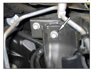
18. Remove the front fender mounting bolt shown. **NOTE: This bolt will used in a later step.**
