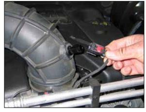
2. Release the red locking tab and then disconnect the Inlet air temperature electrical connection.
