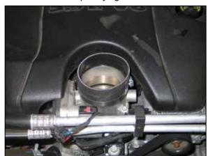
20. Install the provided silicone hose (08698) onto the throttle body and secure with the provided hose clamp.
