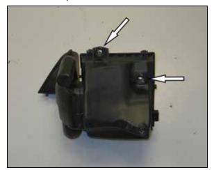
11. Remove two of the factory airbox mounting grommets from the lower airbox.
