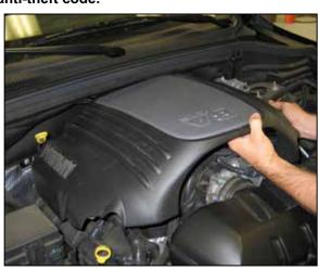
2. Lift up the engine cover to dislodge it from the mounting grommets and remove it from the vehicle.
