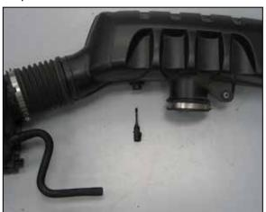
18. Release the locking tab and the remove the inlet air temperature sensor from the factory intake tube by twisting counter clockwise. **NOTE: The inlet air temperature sensor is very fragile; take care to avoid damage while handling the sensor.**
