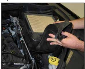
9. Lift up the lower airbox to dislodge it from the mounting grommets and then remove the lower airbox from the vehicle.
