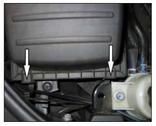
6. Release the two upper airbox retaining clips.
