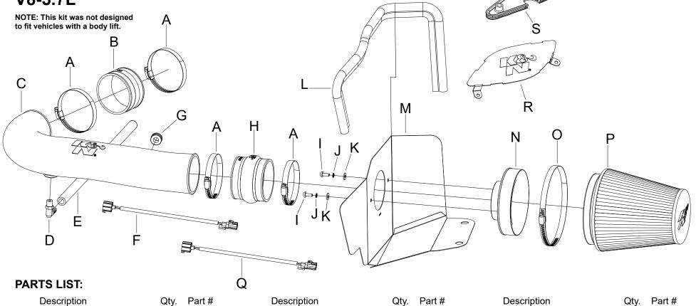
INTAKE TUBE; (IH) BOLT; M6 X 1 X 16MM, BTNHD VENT; 90DEG, 1/2"HOSE, 1/4"NPT, BLK 08110FK WASHER; 6MM FLAT 08269 Ρ AIR FILTER RU-3101HBK **EXTENSION HARNESS** HOSE; 1/2"ID X 19"L 084075 WASHER; M6, SPLIT LOCK 1-3025 21681 Q **EXTENSION HARNESS** EGDE TRIM; (30"L) **BLOCK OFF** 073262 21680 102489 R BLOCK OFF; HOOD VENT, EPDM 21597
