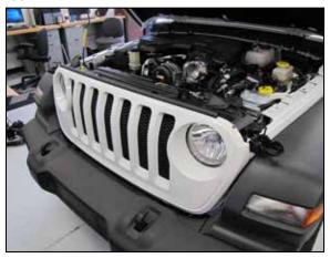
10. Reinstall the grill reengaging the lower clips one at a time then reinstall the six clips that hold the grill to the top of the core support.
