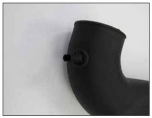
13. Remove the inlet air temp sensor from the factory inlet tube. Then remove the "O" ring from the sensor. Install the provided grommet onto the K&N intake tube. Then install the inlet air temp sensor into the grommet.
