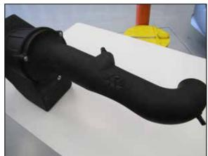
15. Install the K&N intake tube assembly onto the K&N airbox with provided hardware. **NOTE: the**
