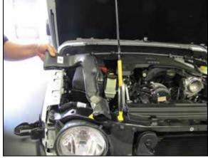
8. Remove the two bolts that secure the inlet scoop to the core support and remove inlet scoop.
