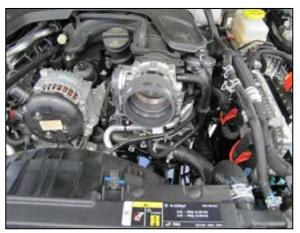
16. Install provided hose onto the throttle body (08171) secure with provided clamp.
