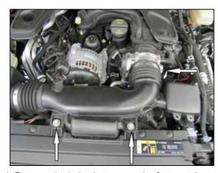
4. Remove the bolts that secure the factory tube to the fan shroud, then loosen hose clamp at throttle body.
