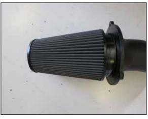
14. Install the K&N air filter onto the K&N intake tube.
