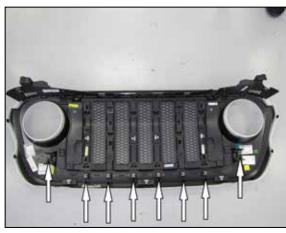
6. Remove the 6 clips at the top of the grill that secure grill to core support. Before removing grill note the location of the 8 clips that hold the lower part of the grill to the core support. Start at either side of the grill. Grasp the bottom part of the grill pulling firmly straight back dielodging the clips one
