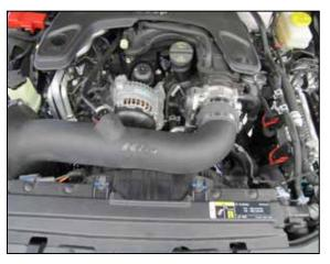
18. Reconnect the crank case vent line onto the quick connect fitting and reconnect the inlet temp sensor electrical connector onto the temp sensor.
