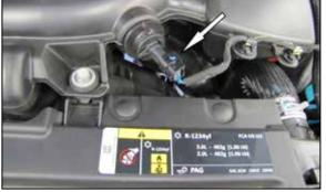
2. Disconnect the inlet air temp electrical connector.
