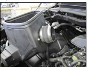
10. Install the provided hump coupler (08418) onto the filter adapter and secure with the provided hose
