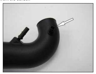
13. Install the sensor into the K&N intake tube using the provided grommet.
