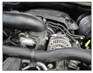
3. Loosen the hose clamp that secures the factory intake tube to the throttle body and then disconnect the intake tube from the throttle body.
