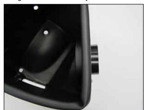
6. Install the filter adapter into the K&N air filter housing and secure with the provided hardware.
