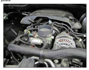
9. Install the provided coupler (08698) onto the throttle body and secure with the provided hose clamp.
