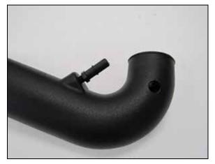
11. Install the provided quick disconnect fitting into the K&N intake tube as shown.
