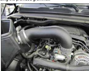
14. Install the K&N intake tube into the hump coupler at the filter adapter and then into the coupler at the throttle body, adjust the tube for best fit and then secure with the provided hose clamps.
