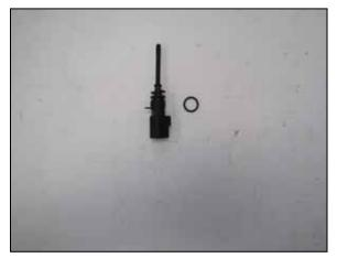
12. Remove the inlet air temperature sensor from the factory intake tube and then remove the O-ring from the sensor.
