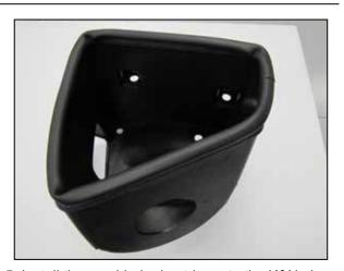
5. Install the provided edge trim onto the K&N air filter housing as shown. NOTE: Some trimming of the edge trim will be necessary.
