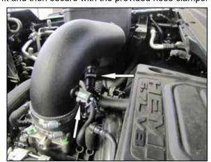
15. Reconnect the inlet air temperature electrical connection. Connect the factory crank case vent line to the quick disconnect fitting installed into the K&N intake tube.
