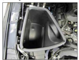
8. Install the K&N air filter housing into the vehicle so the grommets fit onto the factory mounting posts.
