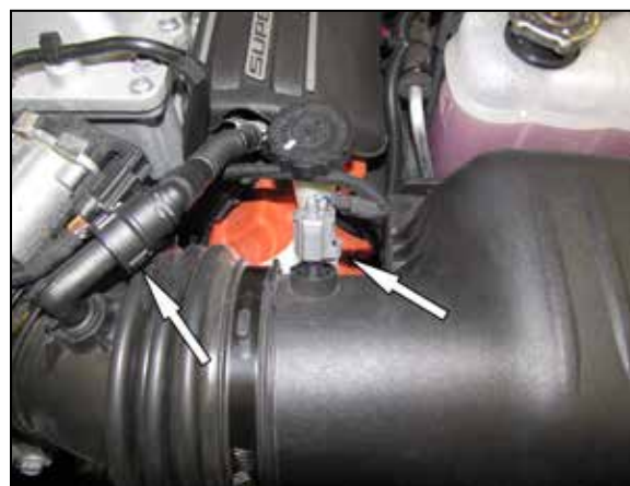
2. Disconnect the inlet air temperature sensor electrical connection and disconnect the crank case vent hose from the fitting.
