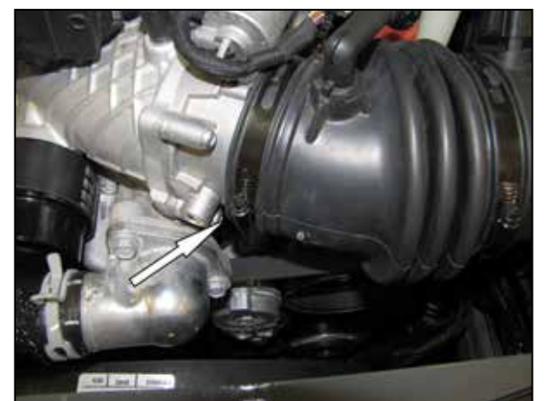
3. Loosen the hose clamp securing the intake tube to the throttle body.
