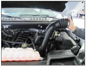
4. Unhook the coolant line from the intake tube and then remove the intake tube from the vehicle.
