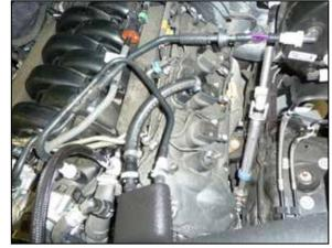
17. On some later models it may be necessary to assemble the crank case vent hose assembly with the provided parts and install due to the manufacturer changing the position on the valve cover port. Install the assembly with the 90\* fitting attached to the valve cover port.
