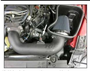
19. Unhook the mass air sensor wiring harness from the inner fender and then route to the mass air sensor and reconnect.
