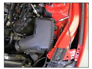
6. Release the clips that secure the upper air filter housing and then remove the upper air filter housing from the vehicle.
