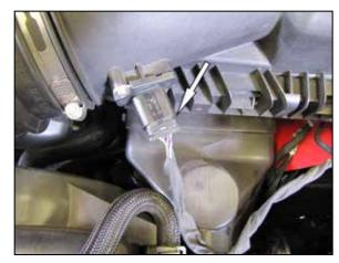
4. Disconnect the mass air sensor electrical connection.
