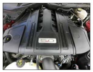
20. Reinstall the engine cover and secure with the factory hardware, reinstall the nut covers. Reinstall the strut tower brace and secure with the factory nuts.
