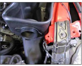
14. Install the filter adapter into the K&N air filter housing and then install the tube gasket onto the adapter. **NOTE: Be sure the threaded inserts in the adapter are aligned with the holes in the housing and gasket.**
