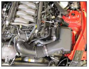
5. Disconnect the EVAP vent line, cut the clamp for the sound tube at the sound drum and disconnect the hose from the drum. Loosen the hose clamps that secure the intake tube to the throttle body and air filter housing then remove the intake tube from the vehicle.
