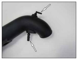
9. Install the provided fittings into the K&N intake tube as shown.
