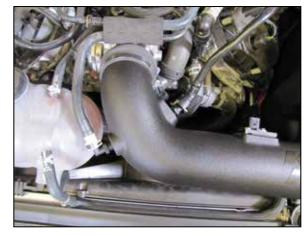
16. Connect the EVAP and crank case vent lines to the fittings installed into the K&N intake tube.
