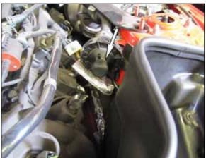
17. Install the provided cap onto the sound drum as shown.
