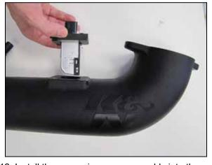
12. Install the mass air sensor assembly into the K&N intake tube as shown and secure with the provided hardware.
