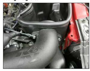
15. Install the intake tube into the coupler at the throttle body and onto the filter adapter, secure the tube to the filter adapter with the provided hardware and to the coupling hose with the provided hose clamp.
