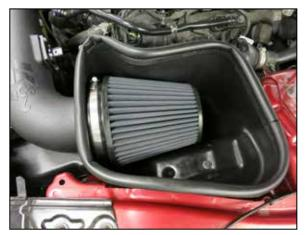
18. Install the K&N air filter onto the filter adapter and secure with the provided hose clamp.
