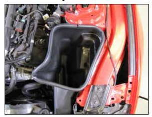
8. Install the provided edge trim onto the K&N air filter housing. Install the K&N air filter housing into the vehicle and secure with the provided hardware. NOTE: Some trimming of the edge trim will be necessary.
