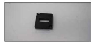
10. Install the provided gasket onto the K&N mass air sensor adapter.
