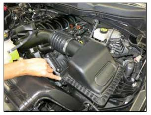
2. Release the two locking tabs that secure the upper air filter housing.
