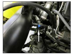
4. Disconnect the CCV from the factory intake tube.
