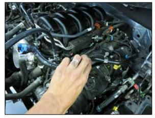
6. Disconnect the CCV line from valve cover.
