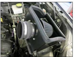
15. Install the provided hump hose onto the filter
