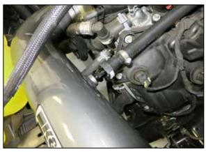
18. Connect the CCV hose to the quick connect fitting installed onto the intake tube.
