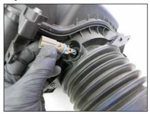
19. Rotate the IAT sensor counterclockwise and up to remove it from the factory air filter housing.
