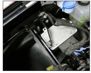
31. Secure the air filter housing to the inner fender with the provided bolt.
