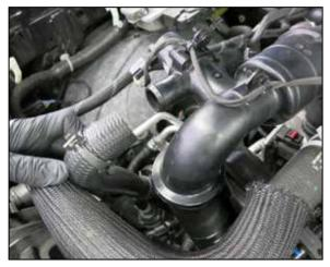
10. Release the spring clamp that secures the BOV hose to the fitting and then disconnect the hose.
