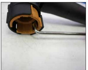
13. Disconnect the CCV hose from the valve cover. There are three clips inside the connector that lock the fitting onto the valve cover, using a 90degree pick the clips can be released one at a time while applying slight pressure upwards on the fitting. The
