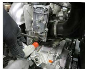
9. Loosen the hose clamp the secures the factory intake tube to the turbo.
