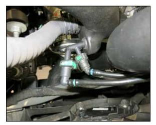
25. Reconnect the Elector hoses onto the ejector installed into the K&N intake tube.
