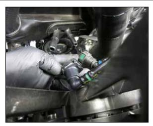
12. Depress the green locking clip on the smaller EVAP hose and then disconnect it from the ejector fitting.
