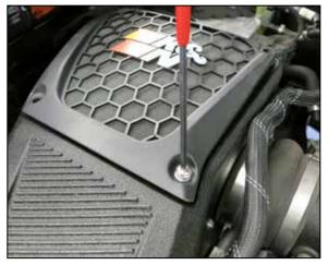
39. Install the prefilter onto the air filter housing and secure with the provided hardware.
