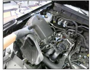
8. Remove the factory air filter assembly from the vehicle.
