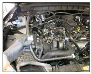
2. Release the CCV quick connect fittings, unhook the CCV line from the radiator fan shroud and then remove CCV line from the vehicle.
