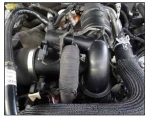
24. Install the BOV hose onto the BOV fitting. Do not secure with the spring clamp currently.
