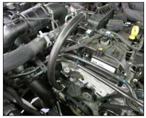
27. Install the CCV assembly onto the quick connect fitting installed into the K&N intake tube and on the valve cover as shown.
