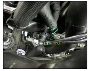
11. Remove the green locking clip that secures the larger EVAP hose to the Ejector fitting and then disconnect the hose.
