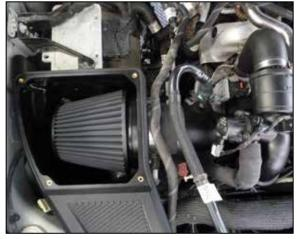
37. Install the K&N air filter onto the filter adapter and secure with the provide hose clamp.
