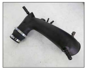
21. Install the provided step coupler onto the K&N intake tube and secure with the provided hose clamp.
