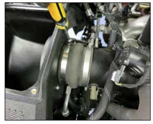
30. Connect the intake tube to the coupler and secure with the hose clamp.
