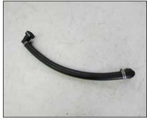
26. Assembly the CCV hose with the provided quick connect fittings as shown.
