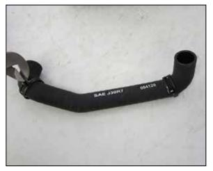
15. Remove the factory BOV spring clamps from the factory BOV hose and install them onto the provided BOV hose.
