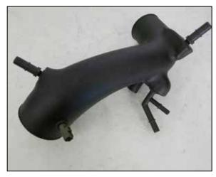
20. Remove the O-ring from the IAT sensor and then install it into the remaining grommet installed into the K&N intake tube.
