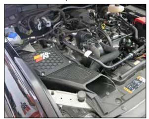
41. Reconnect the negative battery cable. Double check to make sure everything is tight and properly positioned before starting the vehicle. **NOTE:** With the K&N intake system install you will notice more noise from the intake system, turbo charger and blow valve system. You will hear air escaping and the BOV pop on deacceleration. This is normal.
