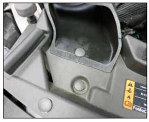
32. Install the factory push-pin to secure the fresh air intake duct.
