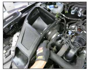
29.Install the K&N air filter housing assembly into the vehicle.
