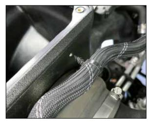
35. Secure the coolant hose to the K&N air filter housing.
