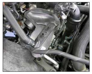
14. Remove the factory intake tube assembly.
