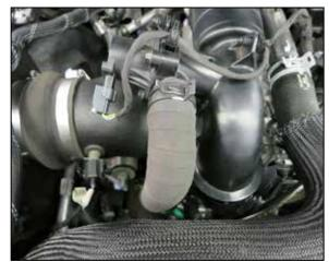
36. Secure the BOV hose to the BOV valve with the factory hose clamp.
