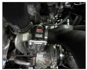
33. Tighten the hose clamp the secures the intake tube to the turbo inlet.
