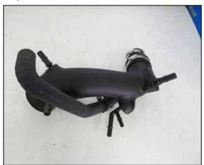
22. Install the provided BOV with factory clamps onto the K&N intake tube.
