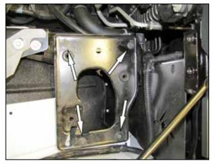
7. Remove the four bolts securing the air box mounting tray and then remove the tray from the vehicle. NOTE: Three of the bolts will be reused in a latter step.
