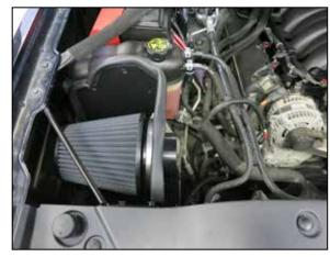
11. Install the filter assembly into the heat shield filter top first, then rotate the filter and pass the adapter through the hole in the heat shield. Secure the filter adapter to the heat shield using the provided hardware.
