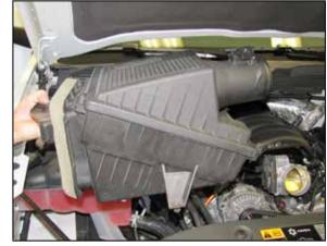
6. Pull up the air box to release it from the mounting grommets and then remove the factory air box from the vehicle. NOTE: It will be necessary to unhook the mass air sensor wiring harness from the air box as it is removed.
