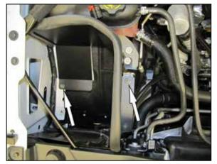
9. Install the heat shield assembly and secure the air box mounting plate location using the three factory bolts from step #7.
