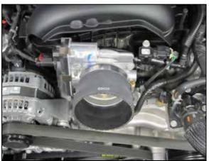
13. Install the coupling hose (08497) to the throttle body and secure with the ded hose clamp.
