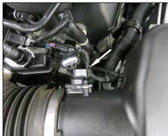
2. Disconnect the mass air sensor electrical connection.
