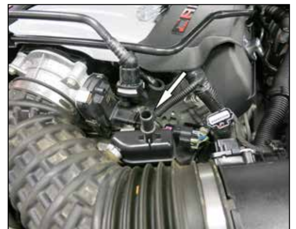
3. Disconnect the crank case vent quick connect fitting from the intake tube.
