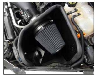
26. Install the K&N air filter onto the adapter and secure with the provided hose clamp.
