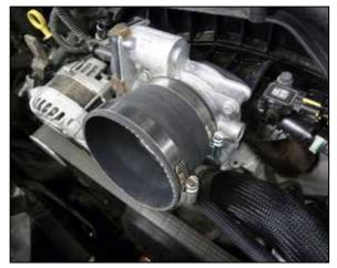
18. Install the provided reducer coupler onto the throttle body and secure with the provided hose clamp. **NOTE: On 5.3L equipped vehicles use coupler #08497, on 6.2L vehicles use coupler #084107**.
