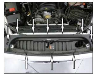
6. Release the ten retaining clips that secure the upper radiator valence and then remove the valence from the vehicle.
