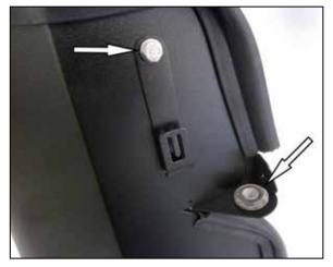
12. Install the provided wiring connector mounting bracket onto the heat shield using the provided hardware. Remove the factory mounting grommet and sleeve from the factory air filter housing and install it into the K&N heat shield as shown.
