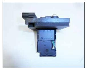
20. Install the provided gasket onto the K&N mass air adapter. Remove the mass air sensor from the factory housing and install it into the mass air adapter and secure with the provided hardware. 24. Connect the crank case vent hose assembly to the valve cover port and then to the fitting installed into the intake tube.
