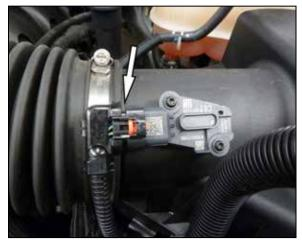
2. Disconnect the mass air sensor electrical connection.
