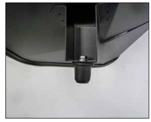
13. Install the provided grommet mount onto the heat shield using the provided hardware and then install the factory mounting grommet onto the mount as shown.
