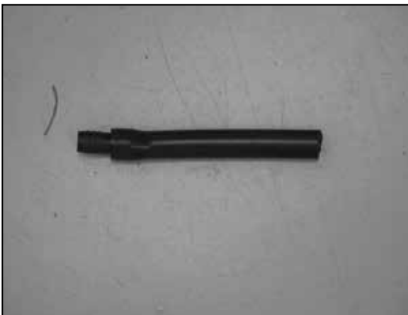
22. Install the hose mender into the provided crank case vent hose as shown.
