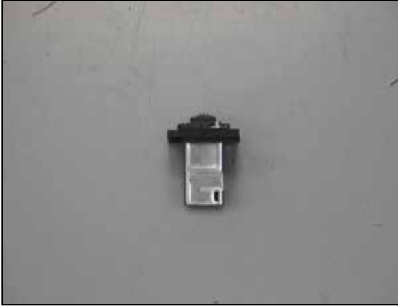
19. Install the mass air sensor assembly into the K&N mass air sensor adapter as shown using the provided hardware.
