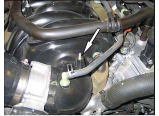
29. Install the provided stud into the mounting stud location as shown.
