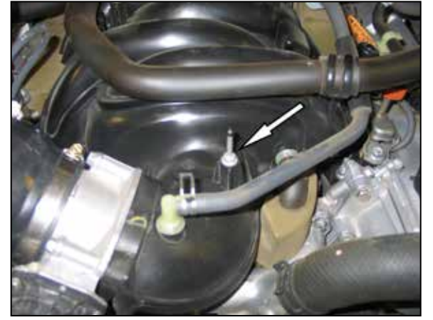
28. Remove the front engine cover mounting stud from the intake manifold.
