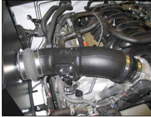
24. Install the K&N intake tube into the hump hose at the heat shield and then into the step hose at the throttle body and secure with the provided hose clamp.
