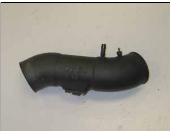
21. Install the provided NPT vent fittings into the K&N intake tube as shown.
