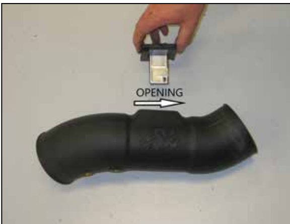
20. Install the mass air sensor assembly into the K&N intake tube so that the opening in the sensor is towards the filter end of the tube as shown.
