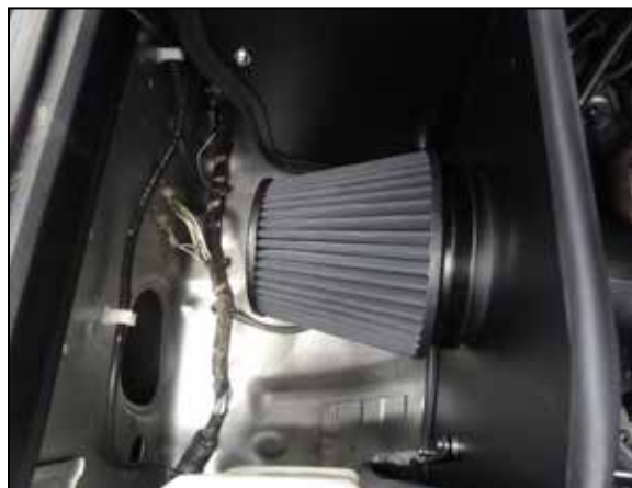
26. Install the K&N air filter and secure with the provided hose clamp.
