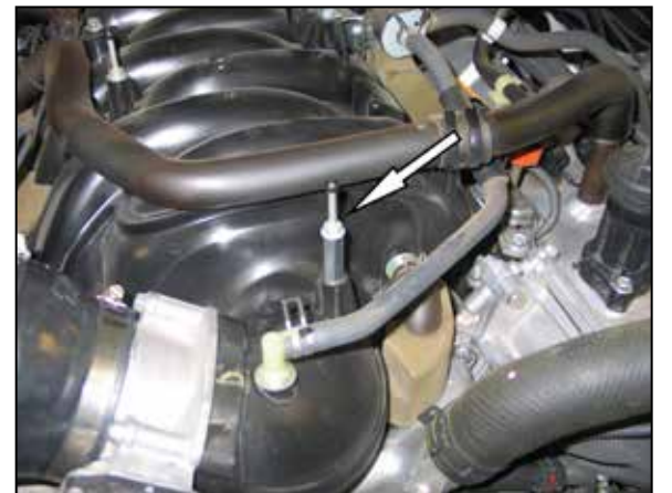
31. Install the mounting stud into the nut extension as shown.
