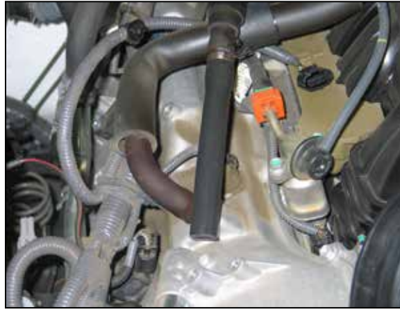
23. Install the crank case vent hose assembly into the factory crank case vent hose as shown.
