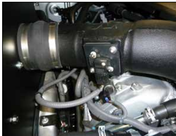
27. Reconnect the mass air sensor electrical connection.
