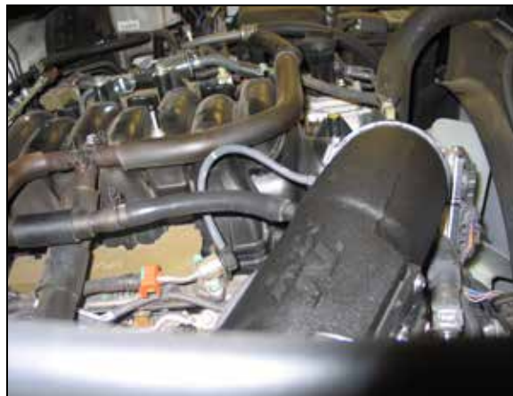
25. Connect the crank case vent hose and the fuel pressure hose to the fittings installed into the K&N intake tube.
