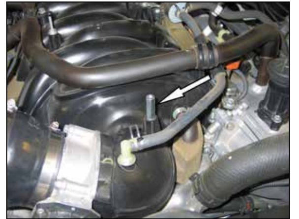
30. Install the provided nut extension onto the stud as shown.
