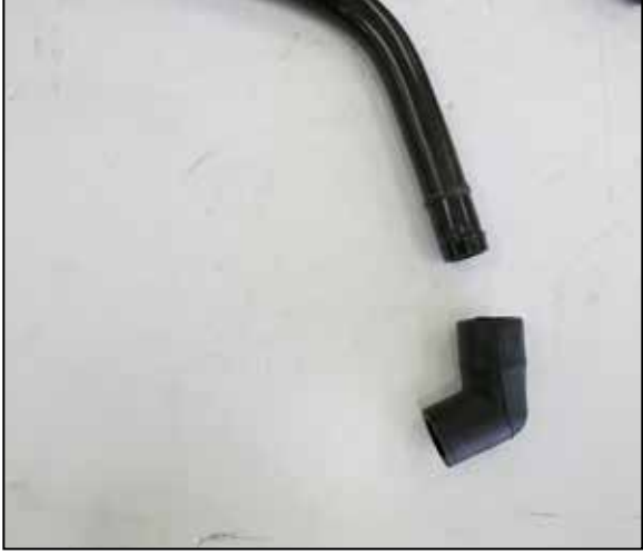
7. Remove the elbow from the plastic hardline.
