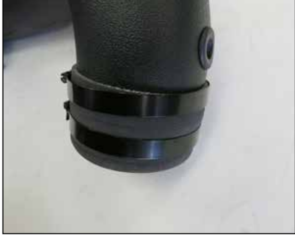
15. Install the provided IAT grommet and coupler hose with clamps. Tighten clamps using 5/16" socket or nut driver. Note: Do not over tighten clamps.
