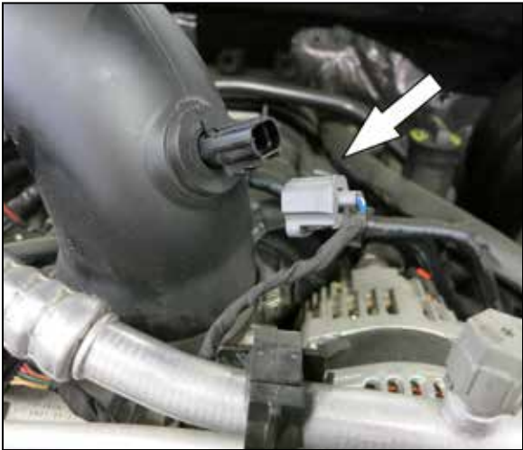
2. Disconnect the IAT sensor electrical connection.
