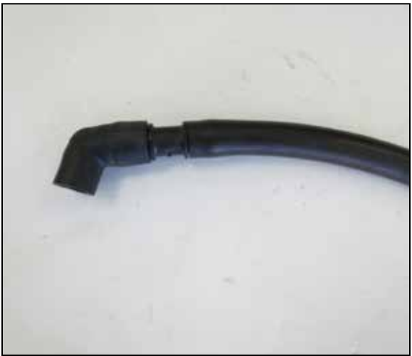
8. Assemble the provided CCV hose, union fitting and factory CCV elbow as shown.
