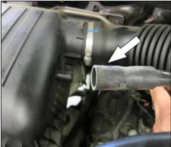
3. Disconnect the CCV hose from the upper air filter housing.
