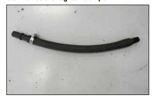
9. Assemble the provided CCV hose, fittings & clamp as shown.
