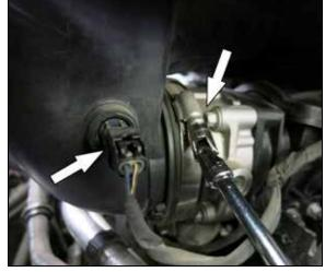
2. Disconnect the IAT sensor electrical connection and loosen the hose clamp that secures the intake plenum to the throttle body.
