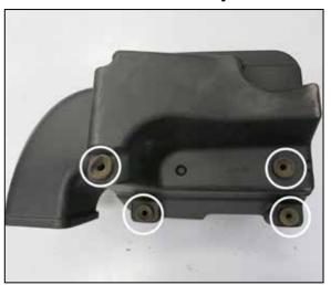
6. Remove the four mounting grommets from the factory air filter housing and install them into the K&N air filter housing.
