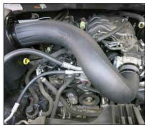
14. Install the intake tube into the air filter and then into the coupler on the throttle body, adjust the tube for best fit and secure with the hose clamps. Tighten clamps using 5/16" socket or nut driver. **Note: Do not over tighten clamps.**
