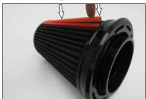
8. Attach the filter clips to the pleats on the air filter align and push down. Passenger side filters, place orange clip on top and red on bottom.
