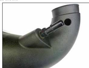
10. Install the provided guick disconnect fitting into the K&N intake tube as shown.
