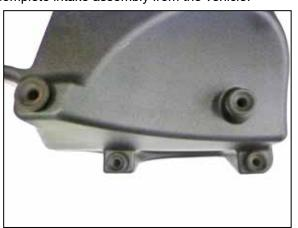
5. Remove the four mounting grommets from the factory air filter housing and install them into the K&N housing as shown.
