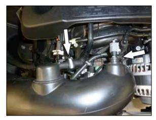
2. Disconnect the crank case vent line quick disconnect fitting. Disconnect the inlet air temperature sensor electrical connection.
