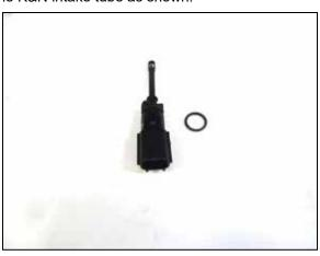
11. Remove the inlet air temperature sensor from the factory intake tube and then remove the O-ring from the sensor.
