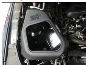
6. Install the K&N air filter housing into the vehicle so the grommets fit onto the factory mounting posts.
