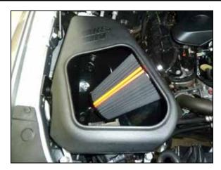
9. Install the K&N air filter into the air filter housing as shown.
