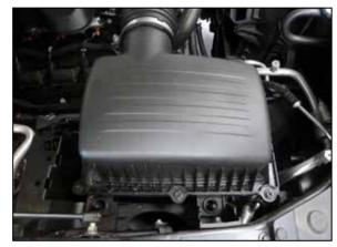
4. Pull up the factory air filter housing to dislodge it from the mounting grommets and then remove the complete intake assembly from the vehicle.
