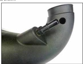
10. Install the provided quick disconnect fitting into the K&N intake tube as shown.
