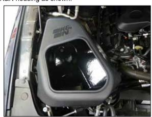
6. Install the K&N air filter housing into the vehicle so the grommets fit onto the factory mounting posts.
