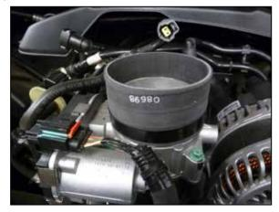
7. Install the provided coupler (08698) onto the throttle body and secure with the provided hose clamp. Tighten clamps using 5/16" socket or nut driver.
