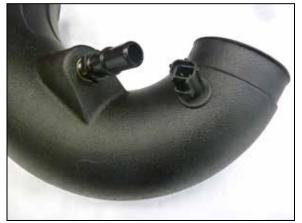
12. Install the sensor into the K&N intake tube using the provided grommet.
