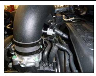
14. Reconnect the inlet air temperature electrical connection and CCV hose.
