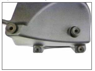
5. Remove the four mounting grommets from the factory air filter housing and install them into the K&N housing as shown.
