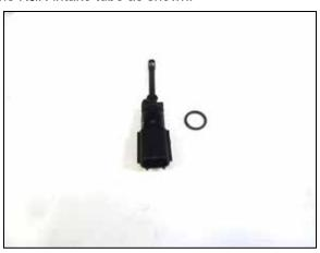
11. Remove the inlet air temperature sensor from the factory intake tube and then remove the O-ring from the sensor.
