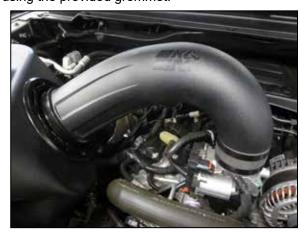
13. Install the K&N intake tube into the filter and then into the coupler at the throttle body, adjust the tube for best fit and then secure with the provided hose clamp. Tighten clamps using 5/16" socket or nut driver.
