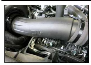
16. Install the K&N intake tube assembly into the air filter and then into the coupler, the coupler will need to flexed around the tube. Align the tube for best fit and then secure with the hose clamps.
