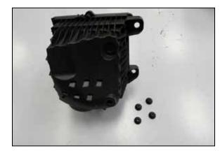
9. Remove the four mounting grommets from the factory air filter housing.
