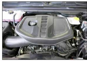
19. Reinstall the engine cover and secure with the factory mounting bolt.
