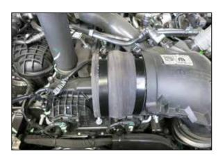
15. Install the provided hump coupler onto the intake plenum with the provided hose clamp.
