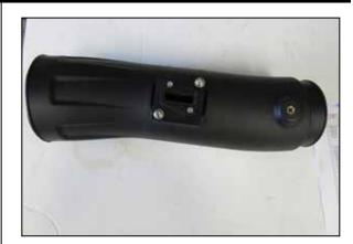
12. Install the provided mass air sensor mounting adapter onto the K&N intake tube using the provided hardware and gasket. NOTE: be sure to install the mounting plate in the position in the photo so the sensor is installed in the correct direction.
