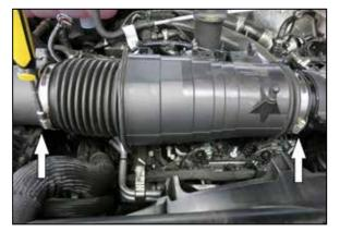
5. Loosen the hose clamps that secure intake tube to the air filter housing and intake plenum.
