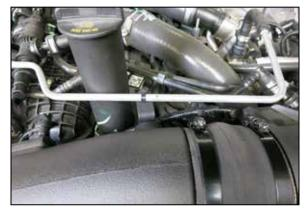
18. Secure the coolant by-pass line to the bracket with the provided mounting cable tie.
