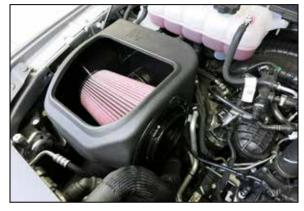
11. Install the K&N air filter into the air filter housing.
