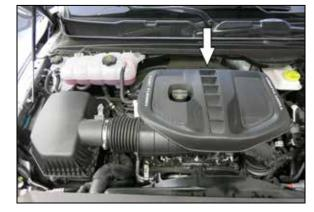
2. Remove the bolt that secures the center of the engine cover then lift the cover up and remove it from the engine.
