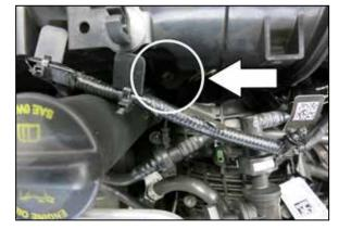
6. Remove the bolt that secures the intake tube to the engine.
