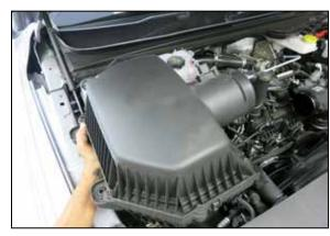
8. Lift the air filter housing up and remove it from the vehicle.
