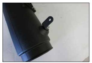
13. Install the provided mounting bracket onto the K&N intake tube using the provided hardware.
