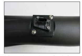
14. Remove the mass air sensor from the factory housing and install it into the adapter installed onto the K&N intake tube. NOTE: Double check to make sure the sensor is installed in the correct direction, the small opening at the bottom of the sensor should be pointed towards the air filter when correct.
