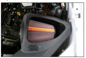
10. Install the air filter into the K&N airbox.
