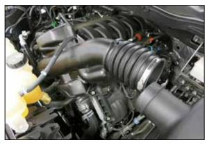
2. Loosen the hose clamp that secures the factory intake tube to the air filter housing. Loosen the hose clamp that secures the intake tube to the throttle body.
