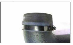
12. Attach the provided hose with clamps to the intake tube. Tighten the clamp on the tube only. NOTE: Verify the throttle body size. Early models will use KITRDCR23 hose and later models will use 08618 hose.
