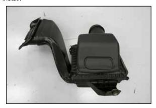
7. Remove the air filter housing/fresh air intake duct assembly from the vehicle.
