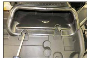
5. Pry up the push-pin locks that secure the fresh air intake duct and remove the pins.
