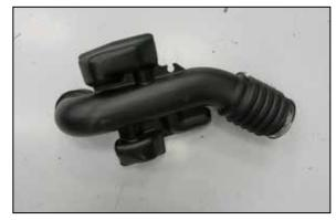
4. Remove the intake tube from the vehicle.
