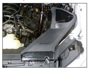
8. Install K&N airbox into factory grommet and position. Secure using original bolt from step 6. Secure the front fresh air intake duct using provided push clips.
