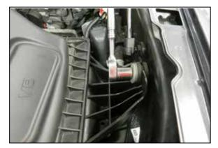
6. Remove the bolt that secures the factory air filter housing to the inner fender. Save bolt for later install.
