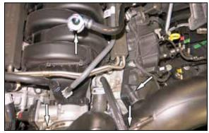
3. Unhook the coolant line and vent lines from the intake tube. NOTE: Early models: Disconnect the EVAP vent connection and crank case vent connection. Later models: Disconnect the crank case vent connection only.
