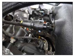
14. Connect the factory CCV hose to the quick connect fitting installed into the K&N intake tube. *NOTE: Early models: Connect the EVAP vent connection.*
