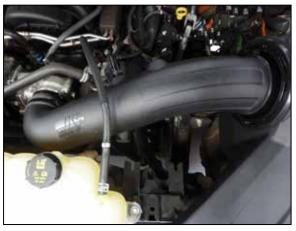
13. Install the intake tube and position the filter and the throttle body. Tighten clamps using 5/16" socket or nut driver. **Note: Do not over tighten clamps.**
