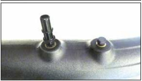
11. Early models: Assemble the 3/8" quick connect and barb fitting with hose like above image. Later models: use provided plastic plug. Install either configuration to the threaded insert on tube. Install the Larger Quick connect 3/8" npt to the threaded insert on intake tube.
