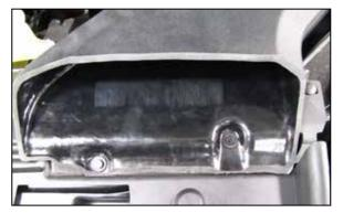
8C. Once the tabs are trimmed flush with the fresh air duct the air filter housing can be installed back into position, pushed down and the locking pins installed as intended.
