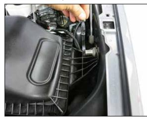
6. Remove the bolt that secures the factory air filter housing to the inner fender and then remove the air filter housing from the vehicle. This bolt will be reused in the next step.
