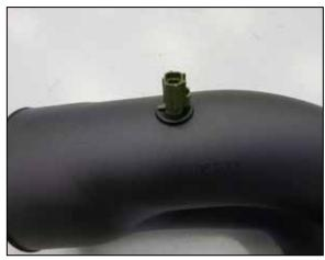
14. Remove the O-ring from the IAT sensor and then install the sensor into the K&N intake tube using the provided grommet.
