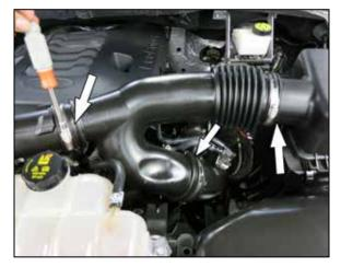
3. Loosen the three hose clamps that secure the factory intake tube.
