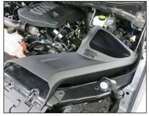
7. Install the K&N air filter housing and secure to the inner fender using the mounting bolt from the
