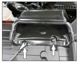
2. Remove the two mounting pins that secure the factory fresh air intake to the radiator valence panel.
