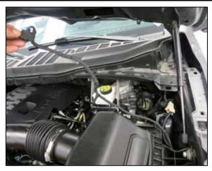
4. Disconnect the IAT sensor electrical connection and unhook the wiring harness from its mounts.
