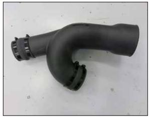
15. Install the provided couplers and clamps onto the K&N intake tube as shown but do not tighten the clamps.Tighten clamps using 5/16" socket or nut driver.
