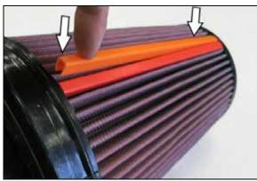
11. Attach the filter clips to the pleats on the air filter align and push down. Driver side filter, place
