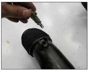
13. Remove the IAT sensor from the factory intake tube.
