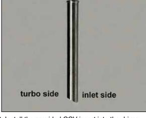
9. Install the provided CCV insert into the driver side inlet tube.
