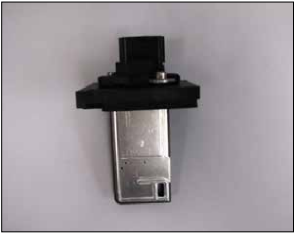
13. Remove the mass air sensor from the factory air filter housing and then install the sensor into the provided adapter using the provided bolts. Install the adapter gasket onto the bottom of the adapter.
