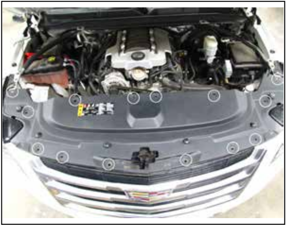
7A. On Cadillac Escalade & GMC Yukon vehicles, remove the fourteen plastic pins that secure the radiator cover and then remove the radiator cover from the vehicle.
