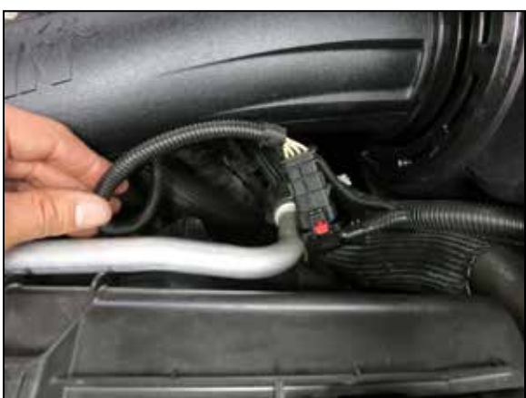
23. Install the crank case hose to the engine and intake tube, make sure you hear the click on the PCV connector.
