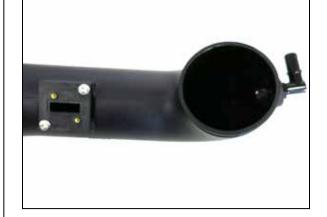
11. Install the provided 90 degree quick connect fitting into the K&N intake tube. Install the provided mass air sensor adapter onto the K&N intake tube using the provided hardware and gasket. NOTE: The quick connect fitting utilizes 3/8npt threads, thread the fitting in by hand and then tighten one revolution. Be sure to install the mass air sensor adapter in the correct
