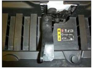
25. Reinstall the hood release arm and secure with the factory hardware.
