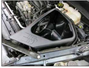
15. Install the airbox into vehicle and position.
