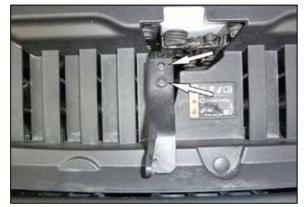
5. Remove the two bolts that secure the hood release arm to the hood latch and then remove the arm.
