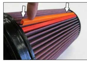
17. Attach the filter clips to the pleats on the air filter align and push down. Driver side filter, place orange clip on top and red on bottom.
