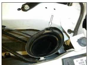
7. Remove the plastic retaining clip that secures the fresh air intake duct to the core support, then
