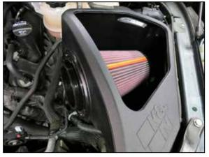
18. Install the air filter into the K&N airbox.
