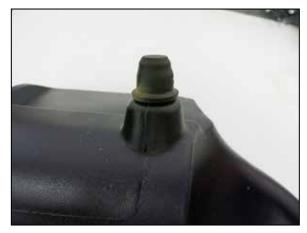
13. Remove the OEM grommmet from the air box and install to the K&N airbox mount ...
