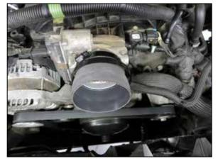
19. Install the 08497 hose to the throttle body with clamps provided for 5.3L models. Install the 084107 hose for the 6.2L models. Tighten clamps using 5/16" socket or nut driver. **Note: Do not over tighten clamps.**
