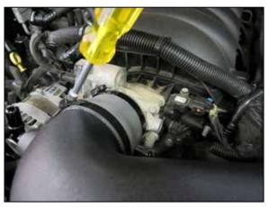
21. Adjust for proper fit, and tighten all clamps.
