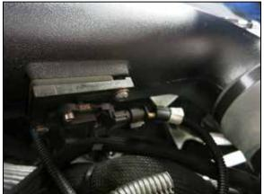
23. Connect the MAF sensor using provided harness extension, and secure harness using cable tie.
