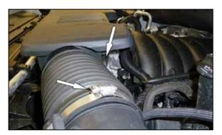
4. Loosen the hose clamps that secures the intake plenum to the air filter housing and to the throttle body. Disconnect the plenum connections at the air filter housing and then rotate the plenum counter clockwise to disengage the keyed mount and separate it from the throttle body.
