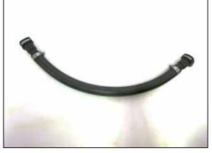
10. Install the provided quick connect fittings into the provided crank case vent hose and secure with the provided hose clamps. Tighten clamps using 5/16" socket or nut driver.
