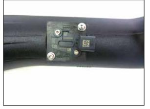
12. Remove the mass air sensor from the factory housing and install it into the K&N adapter using the provided hardware.
