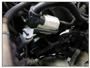
14. Install the provided bracket to the threaded stud air box mount. Slide the bulk connector to the bracket and secure. The K&N airbox will sit on top of this.
