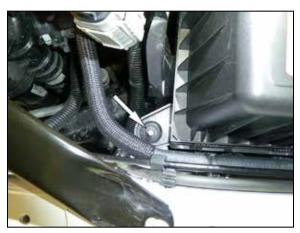
9. Remove the nut that secures the air filter housing. Save for later install. Unhook the wiring harness from the filter housing and then remove the air filter housing from the vehicle. NOTE: Go slow and use caution to remove the housing. It is indexed into two holes in the rear with rubber grommets that can fall off easily and be lost. It is a tight fit but will come out without being forced. These grommets and nut will be reused in later steps.
