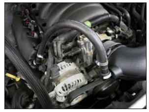
22. Install the crank case hose to the engine and intake tube, make sure you hear the click on the PCV connector.
