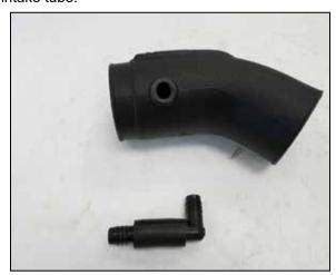
13. Install the provided grommet into the AIRAID intake tube as shown. Assemble the provided CCV fittings and hose in the order shown.
