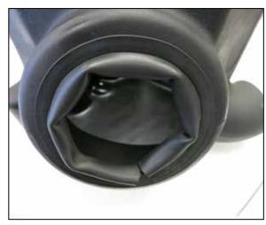
15. Install the provided edge trim into the AIRAID air filter housing as shown. Some trimming of the edge trim will be necessary.
