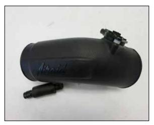
14. Install the CCV assembly into the AIRAID intake tube as shown.
