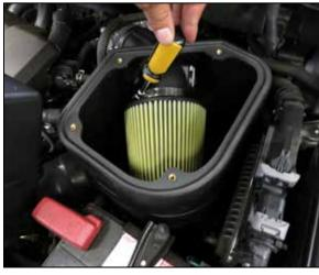
24. Install the AIRAID air filter and secure with the provided hose clamp.
