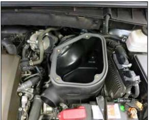
18. Install the AIRAID air filter housing into the vehicle so that the mounting studs protrude through the bottom, secure the housing with the provided hardware.
