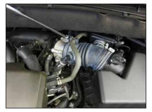
5. Loosen the hose clamp that secures the factory intake hose to the throttle body.
