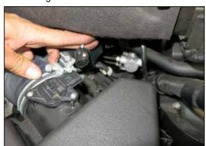
7. Disconnect the mass air sensor electrical connection and separate the harness from the air filter housing.
