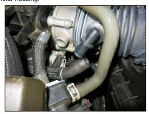
8. Release the spring clamp securing the CCV hose to the factory intake hose and then disconnect the CCV hose from the intake hose.
