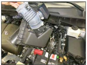
10. Lift up and then remove the complete stock intake system from the vehicle.
