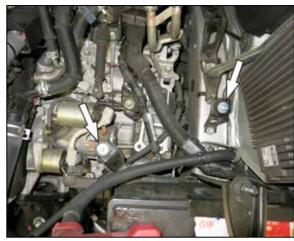
16. Install the two provided rubber mounted studs onto the factory air filter housing mounting locations as shown.
