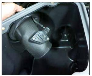
20. Reconnect the mass air sensor electrical connection.
