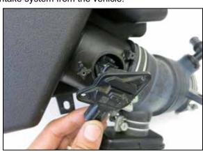
11. Remove the two screws securing mass air sensor and then remove the sensor from the hair filter housing.
