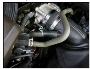
23. Connect the factory CCV hose to the assembly installed into the AIRAID intake tube and secure with the factory spring clamp.
