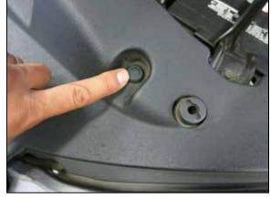
2. Remove the plastic retainer clips that secure the upper valence.
