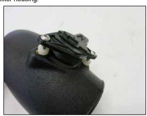
12. Using the two provided spacers, bolts and gasket install the mass air sensor into the AIRAID intake tube.
