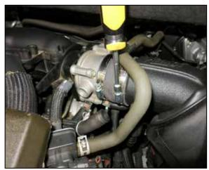
21. Adjust the tube for best fit and then secure with the provided hose clamp.
