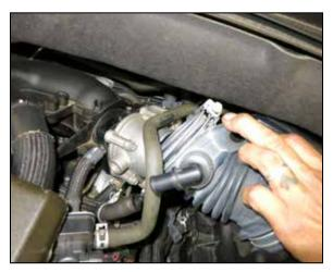
9. Disconnect the intake tube from the throttle body.
