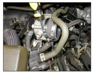
17. Install the provided coupler onto the throttle body and secure with the provided hose clamp.
