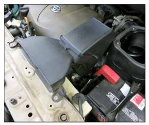
22. Reinstall the factory fresh air duct and secure with the factory hardware.
