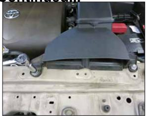
4. Remove the two bolts that secure the fresh air intake duct to the core support.
