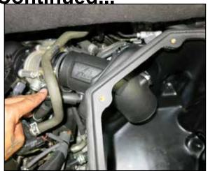
19. Pass the mass air sensor wiring harness through the hole in the air filter housing, then pass the AIRAID intake tube through the air filter housing from the inside and insert it into the coupler on the throttle body.
