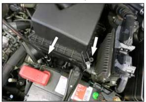
6. Loosen the two bolts that secure the factory air filter housing to the vehicle.
