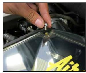
25. Install the air filter housing lid and secure with the provided hardware.
