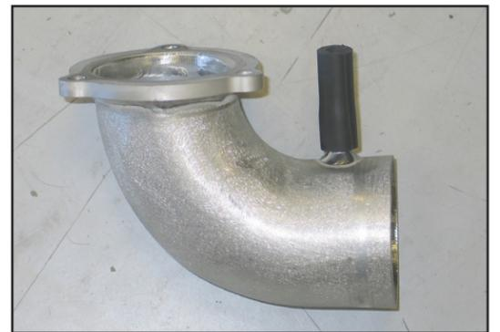
8. Trim the provided crankcase breather hose to a length of 1.5" and then install it onto the K&N® intake tube as shown.
