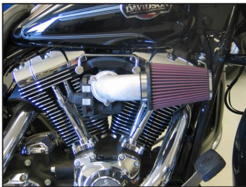
10. Install the provided K&N® air filter and secure with the provided hose clamp. A black hose clamp is being supplied with kit. This clamp is intended to clamp the filter to the intake tube.
