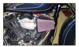
13. Install the K&N<sup>®</sup> air filter onto the intake tube and secure with the provided hose clamp. A black hose clamp is being supplied with kit. This clamp is intended to clamp the filter to the intake tube.
