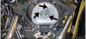
3. Remove the three air filter retaining bolts shown.
