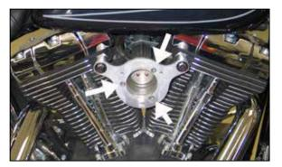
11. Install the provided gasket between the throttle body and back plate and then secure the back plate to the throttle body with the hardware provided. Tighten the crankcase breather bolts. **NOTE: Apply one drop of the provided thread locker onto the provided bolts.**
