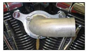
12. Install the K&N<sup>®</sup> intake tube with the gasket and secure with the provided hardware. NOTE: Apply one drop of the provided thread locker onto the provided bolts.
