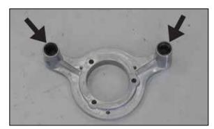
8. Install two of the o rings provided onto the back side of the K&N® back plate as shown.
