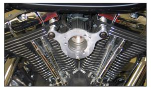
10. Using the two provided crankcase breather bolts; install the back plate onto the vehicle as shown. Do not tighten the breather bolts at this time.
