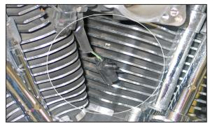
7. Using the provided tie wrap, secure the loose pig tail to the to the throttle position switch wiring harness.
