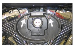
5. Remove the two crankcase breather bolts shown.
