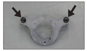
3. Remove the three air filter retaining bolts shown.
