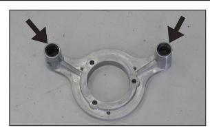
8. Install two of the o rings provided onto the back side of the K&N $^{\mbox{\tiny (8)}}$  back plate as shown.
