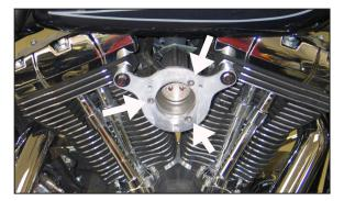
11. Install the provided gasket between the throttle body and back plate and then secure the back plate to the throttle body with the hardware provided. Tighten the crankcase breather bolts. **NOTE: Apply one drop of the provided thread locker onto the provided bolts.**
