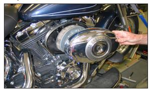
2. Remove the air filter cover retaining bolt and then remove the air filter cover as shown.
