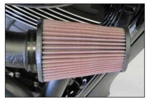
9. Install the K&N<sup>®</sup> air filter and secure with the provided hose clamp.
