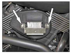
3. Remove the two nuts that secure the bonnet mounting bracket and factory air filter then remove the bracket and air filter.
