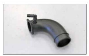
7. Install the provided 90° fitting into the K&N<sup>®</sup> throttle body adapter tube as shown. NOTE: Plastic NPT fittings are easy to cross thread. Install the vent fitting "hand" tight, then turn it two complete turns with a wrench.
