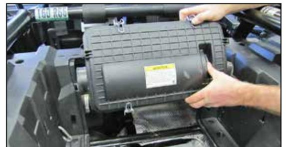
5. Loosen and remove the two hose clamps that secure the fresh air and clean air ducts to the air filter housing. Remove the air filter housing from the vehicle.
