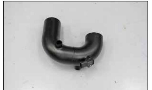
21. Install the inlet temperature sensor into the K&N® intake tube and secure with the provided hardware.
