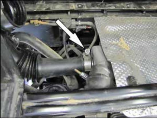
8. Loosen the hose clamp securing the intake tube to the turbo inlet and then remove the tube from the vehicle.
