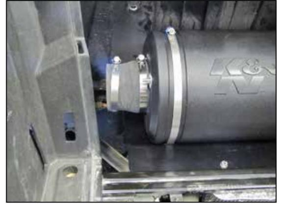
18. Install the provided coupler hose (084055) onto the filter adapter and secure with the provided hose clamp.
