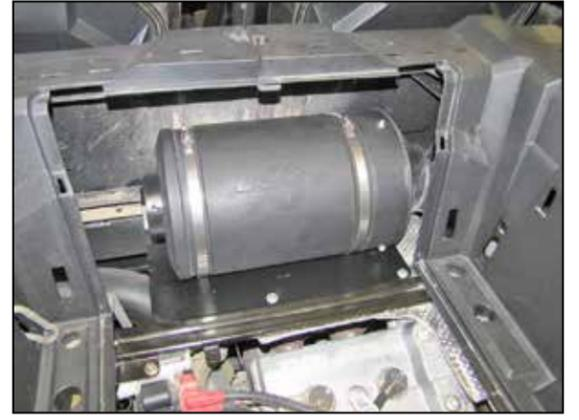
17. Install the filter canister assembly onto the mounting tray and connect the fresh air inlet hose. Adjust the canister and hose for best fit and then secure the canister and hose with the hose clamps.
