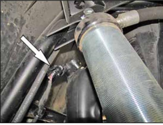
7. Release the clip securing the inlet temperature sensor electrical connection and then disconnect the sensor electrical connection.
