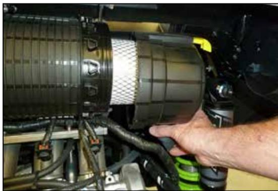
3. Pull out the yellow air filter latch, rotate the air filter housing counter clockwise to unlock and then remove the cover and factory air filter from the vehicle.
