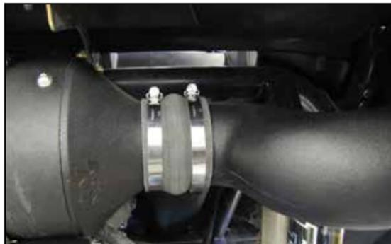
29. Install the provided coupler (08699) onto the Fresh air duct and then install the duct onto the air filter housing but do not completely tighten at this time.
