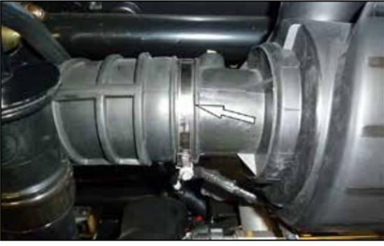
7. Loosen the hose clamp that secures the intake tube to the air filter housing and then disconnect the hose from air filter housing.
