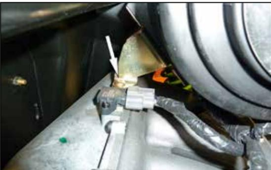
9. Remove the two bolts that secure the air filter housing to the intake manifold using a T30 torx.
