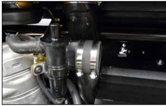
25. Install the provided coupler (08711) onto the K&N® intake tube and secure with the provided hose clamp.
