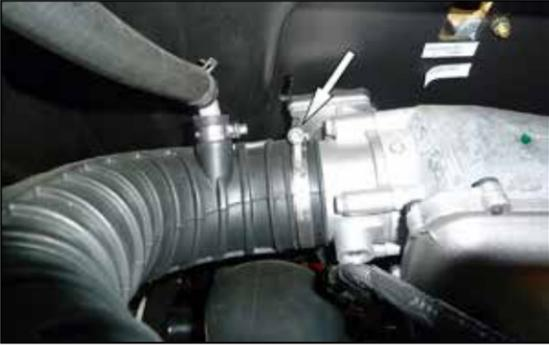
8. Loosen the hose clamp that secures the intake tube to the throttle body and then disconnect the tube from the throttle body and remove the tube from the vehicle.
