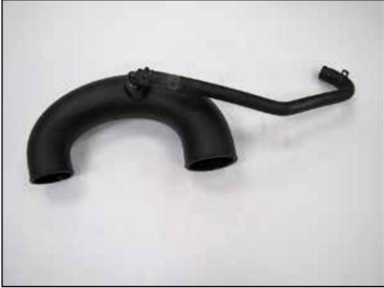
21. Remove the vent fitting from the factory intake tube and install it onto the fitting installed into the K&N® intake tube as shown.
