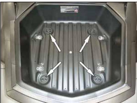
2. Remove the four bolts that secure the cargo tub and then remove the tub from the vehicle.
