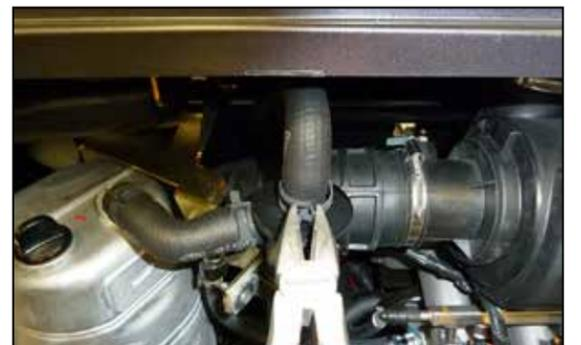
6. Release the spring clamp that secures the breather hose and then disconnect the breather hose.
