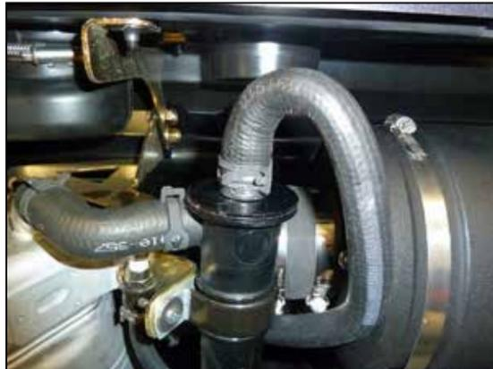
27. Reconnect the vent hose and secure with the factory clamp.
