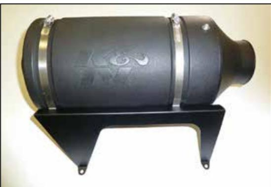
10. Install the K&N® air filter housing lid onto the K&N® air filter housing without the K&N® air filter. Then install the housing onto the mounting bracket and secure with the provided hose clamps as shown.
