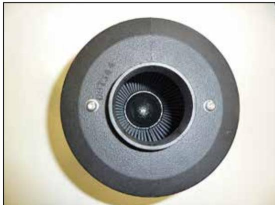
15. Install the filter assembly into the K&N® filter housing and secure with the provided hardware.
