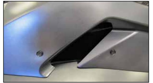
30. Secure the duct to the exterior panel using the provided hardware.
