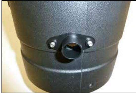
12. Drill two 1/4" id holes for the bolts and one 5/8" id hole for the drain where marked and then secure the drain bracket onto the filter housing.
