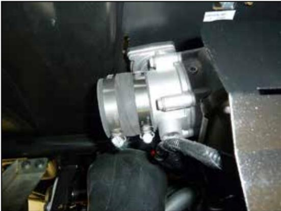
22. Install the provided coupler (5-252) onto the throttle body and secure with the provided hose clamp.
