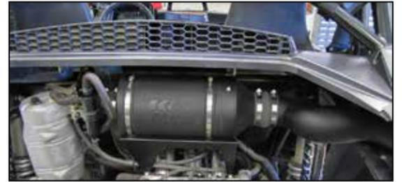
31. Tighten the hose clamps securing the filter housing to the duct.
