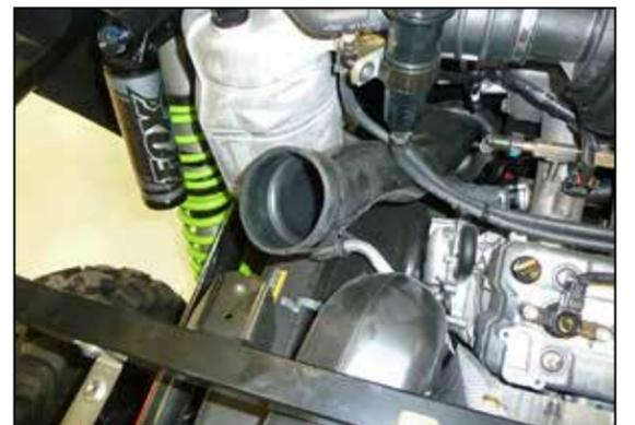
5. Pull the clutch fresh air intake hose down and secure it so that access is achieved for the intake system hose clamps.
