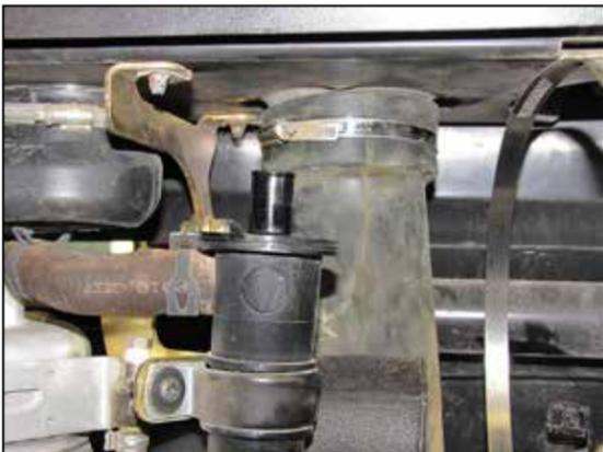
24. Reinstall the clutch fresh air intake hose onto intake and secure with the provided hose clamp.
