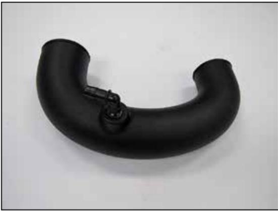
20. Install the vent fitting into the K&N® intake tube as shown.
