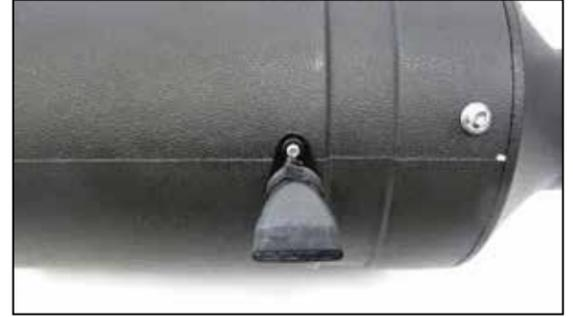
17. Install the duck bill drain onto the drain bracket and secure with the provided tie wrap.
