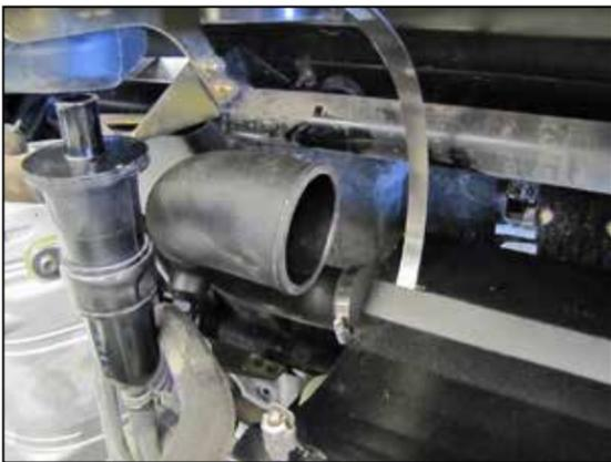
23. Install the K&N® intake tube into the coupler on the throttle body but do not completely tighten at this time.
