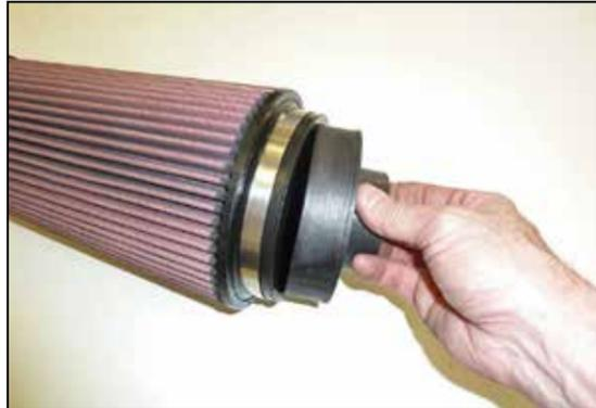
13. Install the filter adapter into the K&N® air filter and secure with the provided hose clamp.
