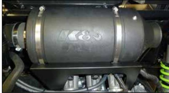
26. Slide the K&N® air filter housing onto the bracket and position so the duck bill drain is through the bracket. Secure the air filter housing with the hose clamps.
