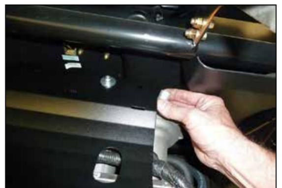
18. Using the bolt, washer and spacers shown, position the air filter housing bracket onto the engine and secure with the bolts to the factory air filter housing mounting locations. Do not tighten the bolts at this time.
