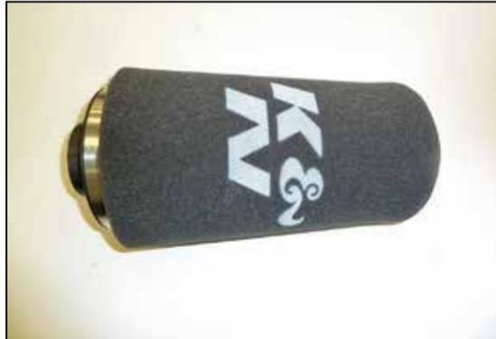
14. Install the K&N® pre-filter onto the K&N® air filter as shown.
