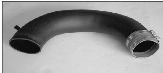
29. Install the provided silicone hose approximately half the length of the silicone hose onto the new K&N® intake tube as shown.
