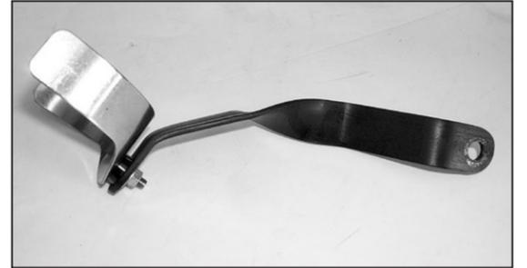
16. Install the new bracket onto the saddle bracket as shown.
