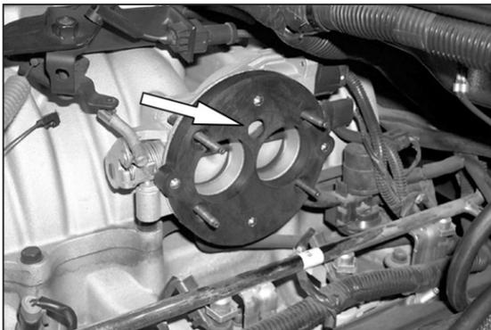
11. Install adapter base plate as shown.
