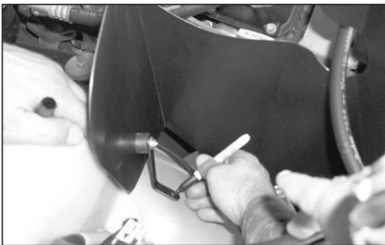
23. Line up the bracket with the inner fender, then mark the hole on the inner fender with a marker or paint pen as shown.
