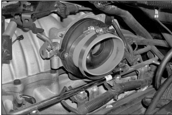
14. Install the provided silicone hose onto the throttle body adapter with the provided hose clamp.
