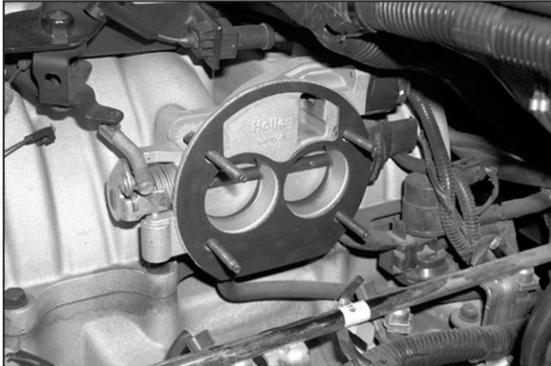
10. Install the provided gasket onto the throttle body as shown.
