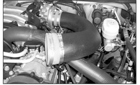
30. Install the new K&N® intake tube onto throttle body as shown.
