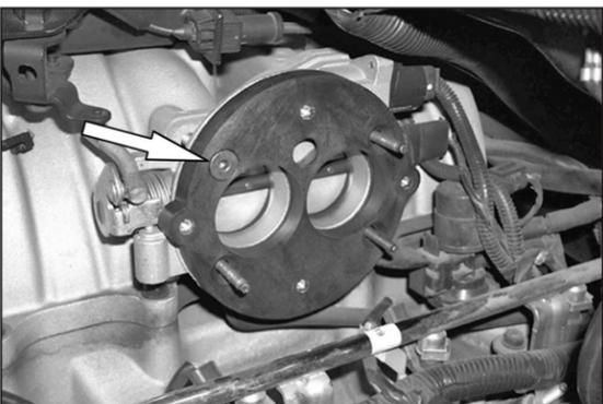
12. One at a time, remove factory studs and install counter sunk allen bolt as shown. Then torque to 30 inch pounds.
