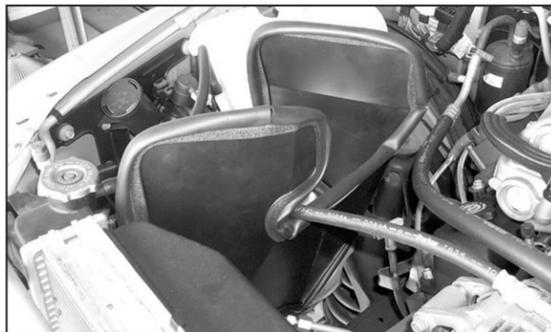
26. Install heat shield onto vehicle then mount using hardware provided.
