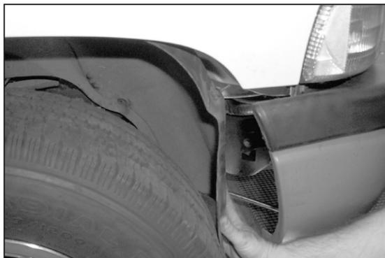
15b. Remove the 3 inner fender mounting retainers by pushing the center release pin in with an 1/8" punch.
