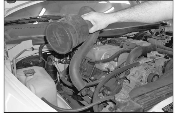
15e. Remove muffler and intake hose assembly from vehicle.
