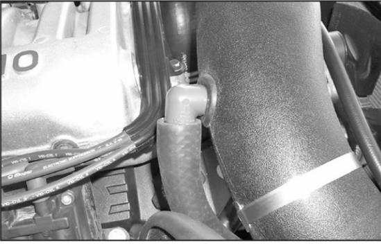
32d. Re-install the intake tube onto the vehicle then install the 90 degree fitting into the grommet on the intake tube as shown.
