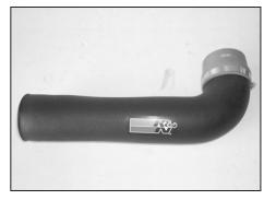
21. Install the silicone hose onto the K&N® intake tube as shown
