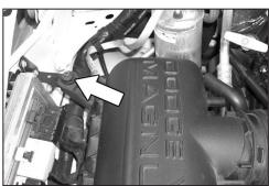
6. Loosen and remove the nut that retains the air box to the vehicle.
