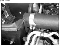
24. Secure the saddle bracket onto the K&N® intake tube with the provided hose clamp as shown.
