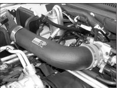
22. Install the intake tube onto the throttle body as shown.
