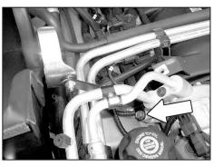
20. Install the saddle bracket assembly onto the A/C compressor with the bolt that was removed in step 19.
