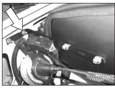
15. Using the nut that was removed in step 13, secure the bracket to the inner fender well.
