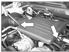
3. Loosen and remove the two bolts that retain the air resonator to the intake manifold as shown.
