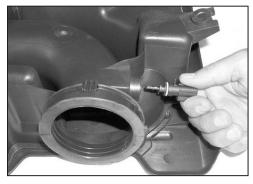
3b. To remove temperature sensor from resonator, turn sensor 1/8 of a turn counter clockwise and remove the sensor as shown.
