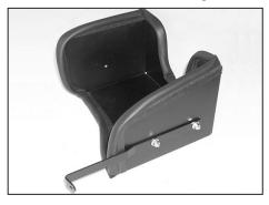
11. Install the provided large "L" bracket onto the heat shield as shown. Do not tighten completely.
