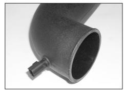
21c. Remove the factory O-ring from the temperature sensor, then install the sensor into the intake tube as shown.
