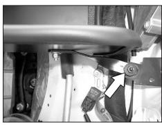
16. Using the nut that was removed in step 6, secure the bracket to the air box mounting stud as shown. Do not completely tighten at this time.
