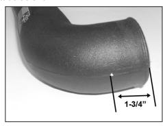
21a. On models that come equipped with an external temperature sensor, mark the intake tube 1-3/4" from the end of the tube, then drill a 3/4" hole into the intake tube.
