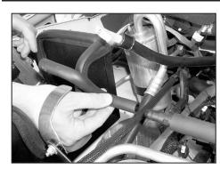
23. Remove the vent hose from the vehicle as shown
