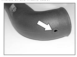
21b. Install the provided grommet into the intake tube as shown
