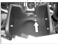
17. Attach the heat shield onto the lower "Z" bracket with the provided hardware.
