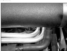
27. Connect the vent hose onto the K&N<sup>®</sup> intake tube as shown.
