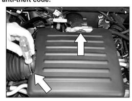
2. Loosen the hose clamp at the throttle body and air intake tube as shown.
