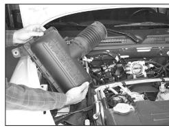
7. Pull firmly upwards on the stock air box to remove from the vehicle as shown.
