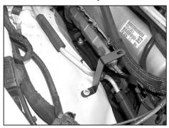
10. Mount the provided "Z" bracket onto the inner fender well as shown. Do not tighten completely.
