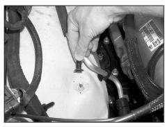
8. Unscrew the plastic air box retaining stud from the vehicle as shown.
