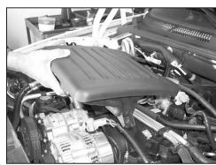
4. Remove the air resonator from vehicle as shown.
