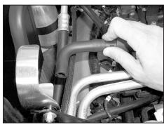
26. Re-install the vent hose onto the vent line as shown.
