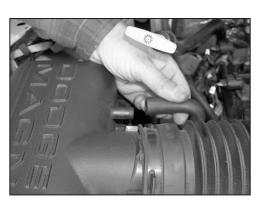
5. Remove the vent hose from the air box as shown.
