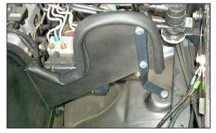
2. Disconnect the crank case vent hose as shown.
