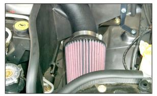
13. Install the K&N<sup>®</sup> Air Filter onto the K&N<sup>®</sup> intake tube and secure with the provided hose clamp. **NOTE: Drycharger<sup>®</sup> air filter wrap; part # RC-4700DK is available to purchase separately. To learn more about Drycharger<sup>®</sup> filter wraps or look up color availability please visit** http://www.knfilters.com<sup>®</sup>.
