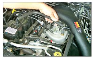
12. Connect the provided hose to the vent on the valve cover, then, connect the other end to the vent on the K&N<sup>®</sup> intake tube as shown.
