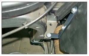
9. Secure the "L" bracket to the hole on the flange/ tab on the radiator core support using the provided hardware.
