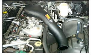
11. Install the K&N<sup>®</sup> intake tube into the silicone hose as shown, but do not tighten completely as some adjustment may be necessary.
