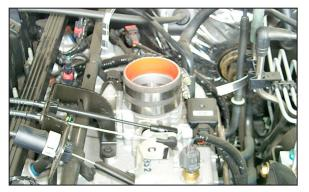
10. Install the provided silicone hose and hose clamps onto the throttle body as shown.
