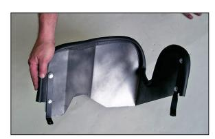
7. Using the provided hardware install the two brackets onto the heat shield as shown.
