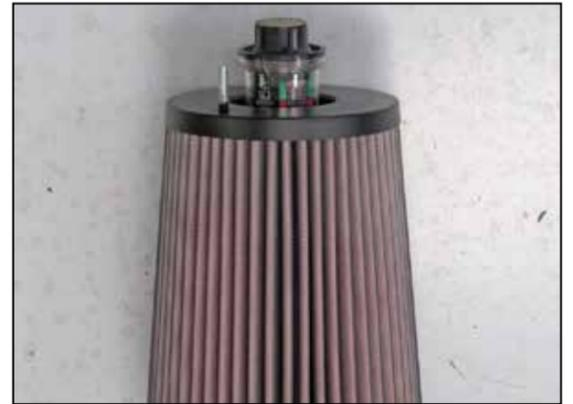
23. On vehicles equipped with a filter minder, install the factory grommet and filter minder into the K&N air filter as shown. On vehicles that are not equipped with the factory filter minder, install the provided plug into the filter.
