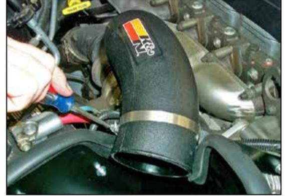
22. Install the intake tube onto the turbo inlet, then align with the saddle bracket. Attach the saddle bracket to the intake tube with the provided hose clamp, adjust the bracket to achieve the appropriate clearance for the intake tube before tightening.
