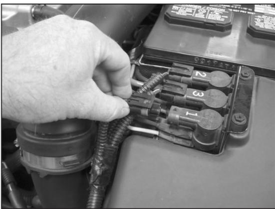
3. Disconnect the three electrical connectors from solenoid pack as shown.
