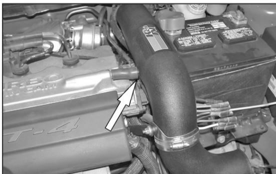
18. Install the K&N® intake tube onto the turbo, then align with saddle bracket. Then tighten all hose clamps.
