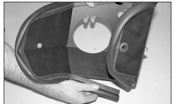
24. Install the edge trim onto the heat shield as shown. Trim if needed.
