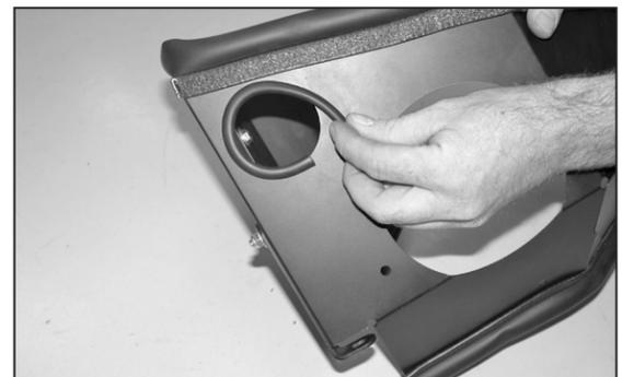
25. Install the edge seal onto heat shield as shown.
