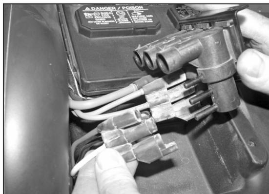
4. Remove the two screws that secure the solenoid pack to air box lid, then disconnect vacuum lines from solenoid pack as shown.
