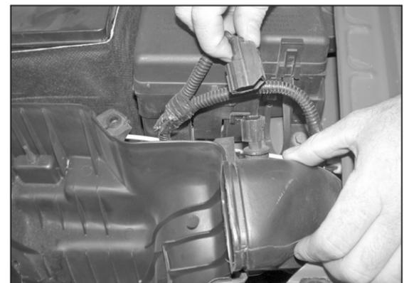
7. Disconnect the air temp sensor electrical connection as shown.
