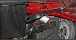
8. Install the twist bracket (070772A) onto the core support using the hardware provided through the existing hole as shown.
