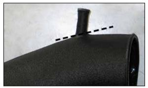
16a. On SRT 8; 6.1L vehicles, cut the vent off of the K&N $^{\circ}$  intake tube as shown.
