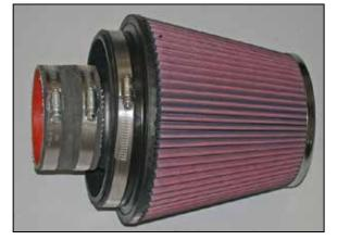
21. Install silicone hose (08630) onto the air filter assembly and secure with the provided hose clamp.
