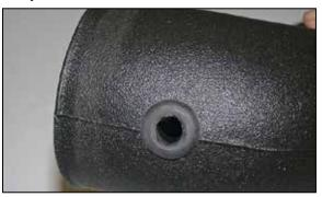
16. Install the provided grommet into the  $K\&N^{\circledast}$  intake tube as shown.
