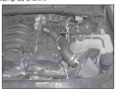
18. Install the K&N® intake assembly into the silicone hose at the throttle body and onto the saddle clamp as shown, then secure with the provided hose clamps. Adjust the air filter assembly for best clearance and tighten the hose clamp, which secures it to the K&N® intake tube.
