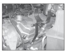
8. Using the provided hardware, install the tubemounting bracket onto the engine at the threaded hole in the cylinder head as shown.
