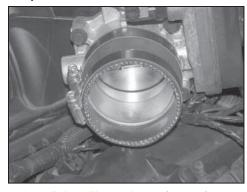
17. Install the silicone hose (08756) onto the throttle body and secure with the provided hose clamp as shown.
