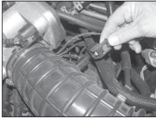
2. Unlock the red locking tab on the air temperature sensor electrical connection, then depress the locking lever and pull apart the air temperature sensor electrical connection.
