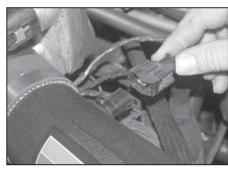
23. Reconnect the air temperature electrical connection as shown.
