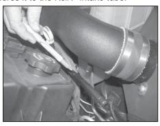
19. Mark the crank case vent tube approximately 1" back from the vent port on the K&N® intake tube as shown.
