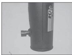
15. Install the air temperature sensor into the grommet installed in step #14.
