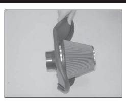
11. Install the K&N® air filter onto the filter adapter as shown.
