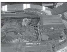
6. Lift the complete intake and air filter assembly to remove it from the vehicle.
