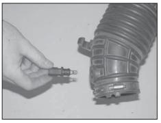
13. Remove the air temperature sensor from the factory intake tube.
