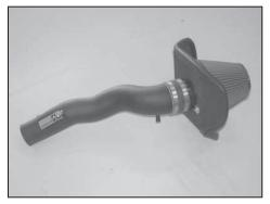
16. Install the air filter assembly onto the K&N<sup>®</sup> intake tube as shown.
