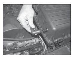
4. Disconnect the crank case vent hose from the airbox as shown.
