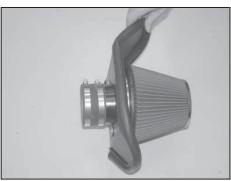
12. Install the silicone hose (08630) onto the filter adapter and secure with the provided hose clamp as shown.
