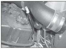
22. Reinstall the crank case vent tube onto the valve cover and then connect to the K&N<sup>®</sup> intake tube as shown.
